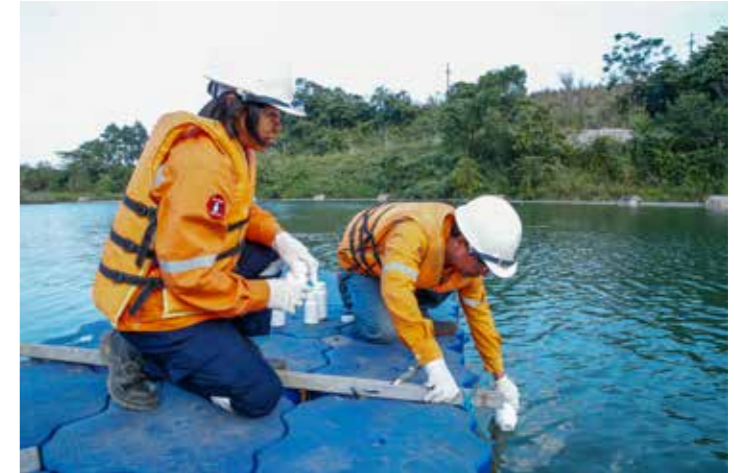
Environmental technicians take water samples in waste water dam of MHT in Vietnam
