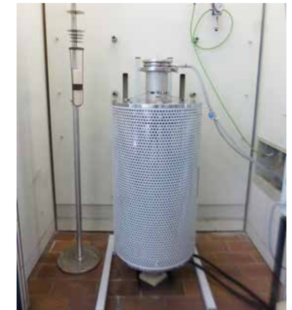
Laboratory Digestion Furnace
