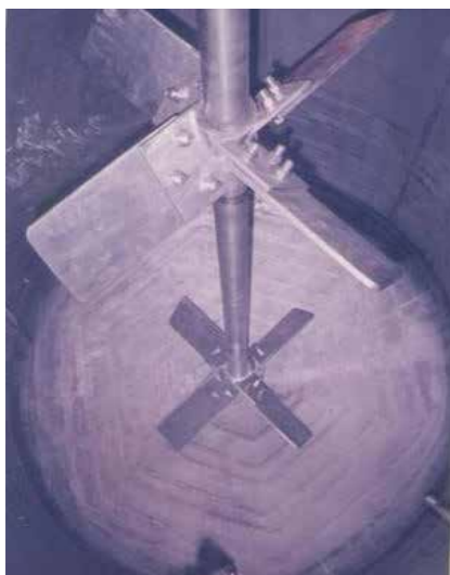
A pitched-blade agitator in the leaching autoclave
