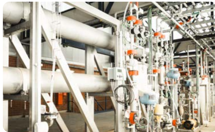
Reverse osmosis equipment in AMT production plant in Goslar/Germany
